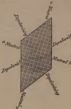
FIG. 19. Imaginary Structure of a Plate of Selenite.
